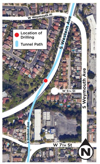
The Sanitation Districts has begun drilling on Western Avenue across from the 5th Street cul-desac, requiring one southbound traffic lane closure. A 4-inch bore hole is being drilled to a depth of 370 feet, so we can investigate conditions in our underground tunnel using a camera. There are no safety issues or concerns for this area while this work takes place.
