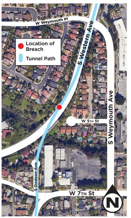
The Sanitation Districts is beginning work on Western Avenue across from the 5th Street culde-sac that requires one southbound traffic lane closure. A 6-inch bore hole will be drilled to a depth of 370 feet so we can investigate conditions near our underground tunnel at this depth. This drilling will allow us to send a remote camera down to our tunnel to examine conditions. There are no safety issues or concerns for this area while this work takes place.
